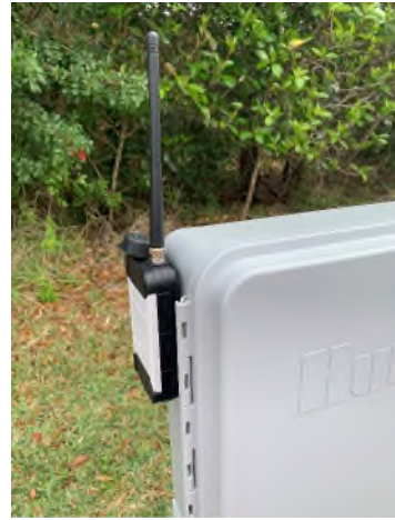
Receiver plugged into Socket on side of Controller
