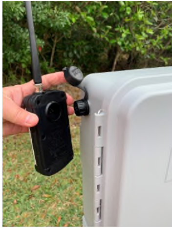
Lift cap and plug Receiver Unit into Socket
